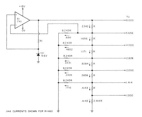
within 0.5% of the calculated ratios, in- 1k, 8.25k and 2.43k. For general use, an suring good accuracy, especially if the op amp and zener diode produce a regulated voltage source. The voltage at If extreme accuracy is required, then the top of the ladder will be 1.41 times the zener voltage. Of course one may connect the ladder to another regulated voltage if one is available.
